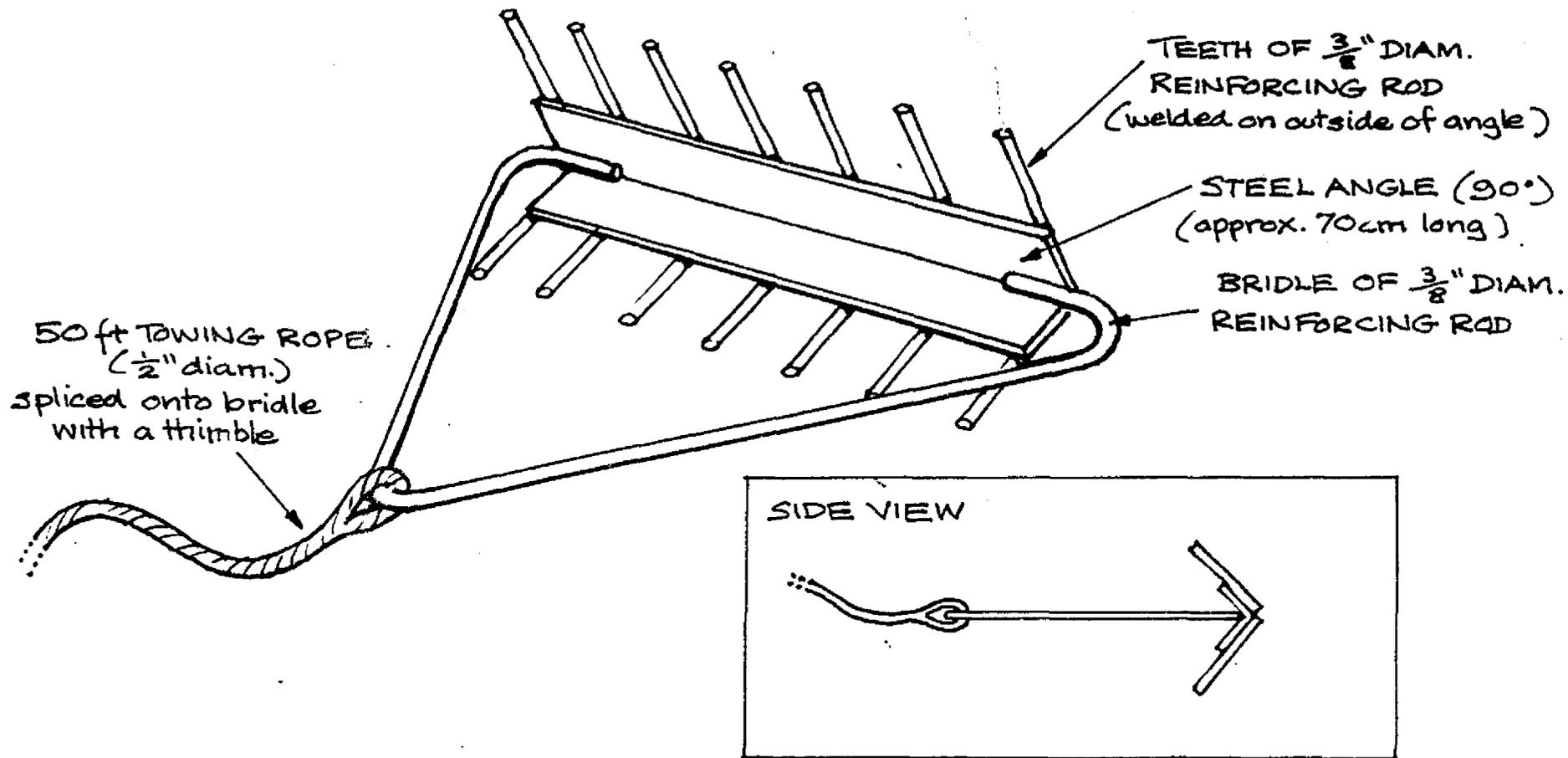
FIGURE 2: A grapnel designed for towing masses of floating aquatic weeds.
