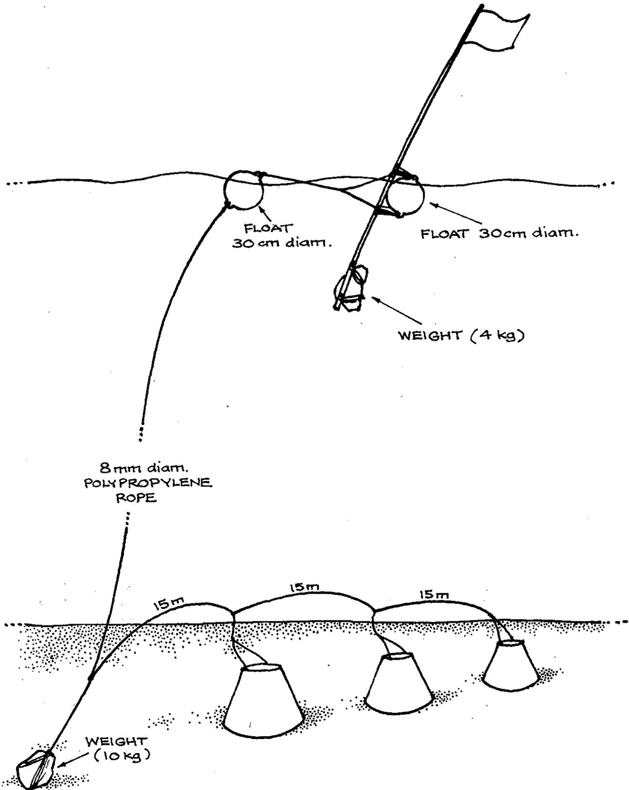
FIGURE 3: The arrangement of the traps used in the survey. The length of dropline used (i.e. between buoys and bottom weight) was equivalent to the depth of water plus a minimum of 25% excess rope.
