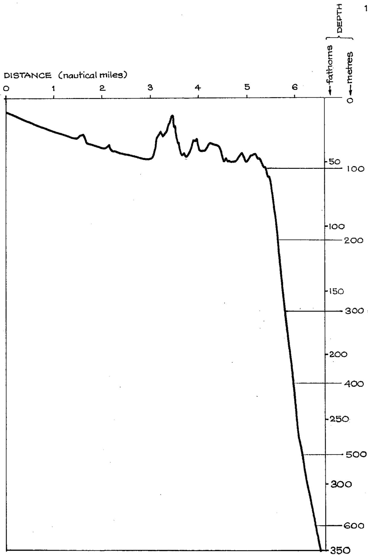
FIGURE 5: The depth profile, measured by an echo-sounder trace, of the transect line indicated in figure 4; i.e. on a bearing of  $14^{\circ}$  TRUE out from Apia harbour
