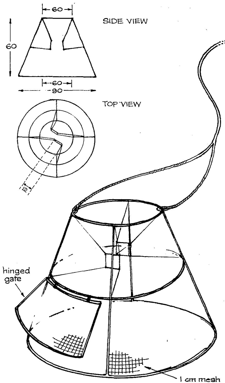
FIGURE 2: The shrimp trap used in the survey. The two entrances were made from the wire mesh (without any frame work) and were offset (see top view) so that the inner openings were not directly opposite each other. Drawings not to scale; measurements given in centimetres.
